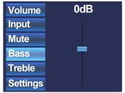
The other settings which can be changed to the zone is the two band tone control. The tone control can be activated by selecting the 'Bass' and 'Treble' buttons, and the adjustment of the tone control works with a fader just as the volume control. You can increase and decrease the high and low tones the same way as adjusting the volume, by simply rotating the selection dial. The Bass and Treble both can be adjusted between the ranges of +14dB and -14dB
