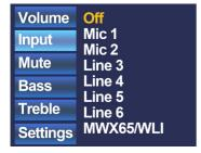
When 'Input' is lit, you can push this button and you will be redirected to the input selection window. This window shows all (configured) input channels which can be selected. You can scroll through the inputs by rotating the selection dial, and the desired input can be selected by pushing the dial.
