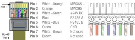
Below is the cable connections when using two MWX65 units on a single wall panel input using a single CAT5e cable.
