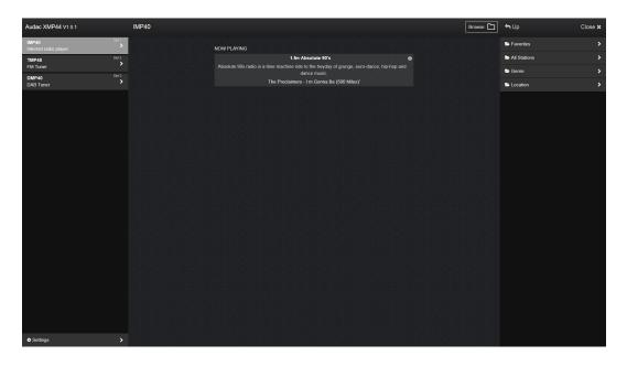
The modules screen gives an overview of the controllable functions for the currently selected module. The currently selected / controlling module is highlighted in the left side column and the main area (center) of the screen indicates the current operation mode, depending of the offered functionalities for the installed module.
