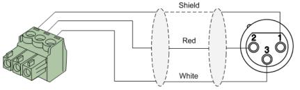
For unbalanced line in & output connections:
