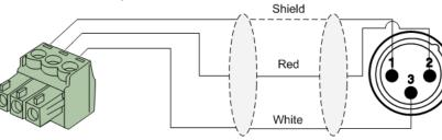
For balanced line output connections:
