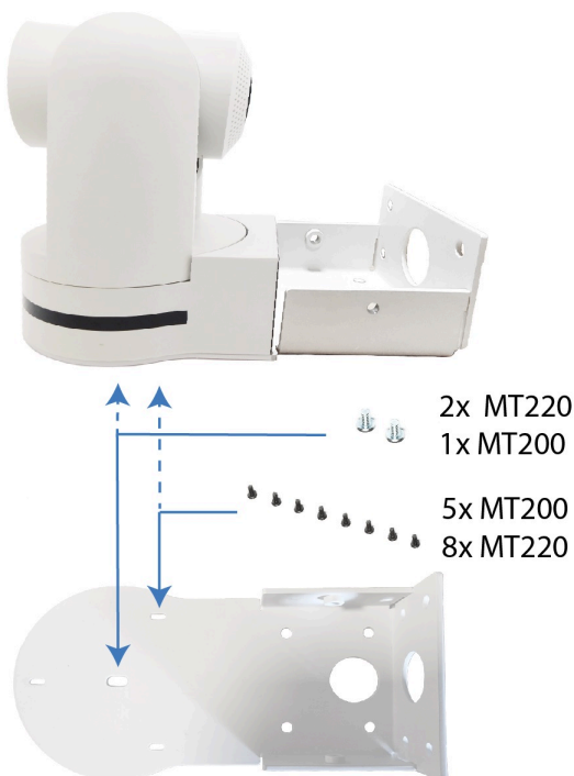
Figure 3: Mounting camera to the baseplate
