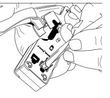
Roll up the drain wire and place in the base of the external ground. As you start to bring the external ground into place onto the cable, keep the mass of drain wire tucked in so it is totally covered.
