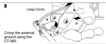
Use the large or small tool cavity depending on the size of your cable.
