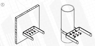
Remove the "U" bracket from the speaker. Drill the mounting location holes for the unit in line with the "U" bracket (2 holes 30 mm apart) in the surface where the loudspeaker is to be located.
