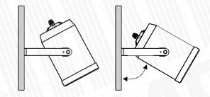
Re-fit the speaker to the "U" bracket. Position the speaker to the desired angle, then tighten the fixings to secure in place.
