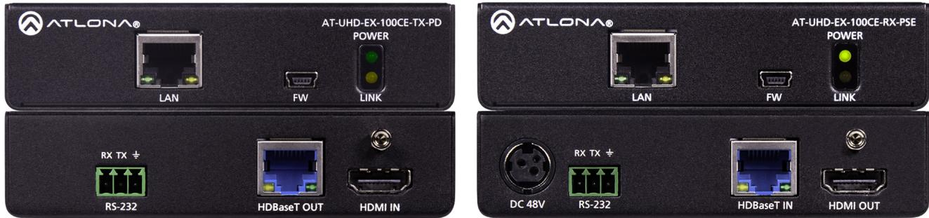
The Atlona **100CER-PoE-EXT** is an HDBaseT™ transmitter and receiver combination that includes the **AT-UHD-EX-100CE-TX-PD** HDBaseT transmitter and **AT-UHD-EX-100CE-RX-PSE** HDBaseT receiver. It extends HDMI up to 330 feet (100 meters) over category cable with Ethernet pass-through and RS-232 control. The 100CER-PoE-EXT supports video signals up to 4K/UHD @ 60 Hz with 4:2:0 chroma subsampling, plus embedded multi-channel audio.
