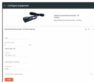
20 Select edit on the controlled device's tile. A new window will slide open.
