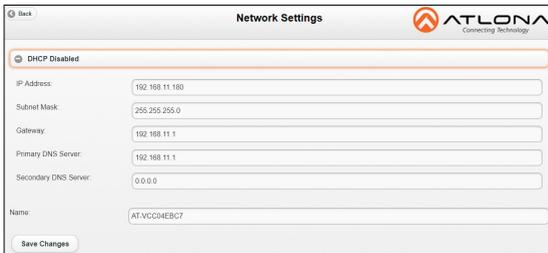
9 Type in the IP details to match the network details of the Gateway. e.g. If the Velocity gateway is located at the IP of 192.168.12.15, then the VCC should be set to an IP within the 192.168.12.XXX range that has not already been used.
