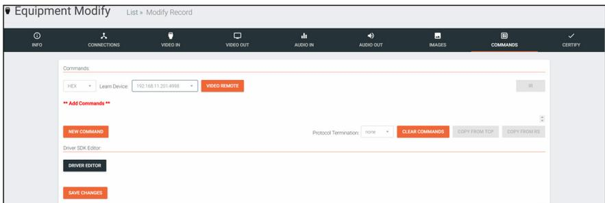
13 Press the NEW COMMAND button. A new line will appear above the button.
