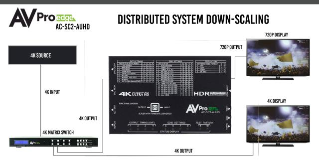
WITH THE AC-SC2-AUHD YOU ARE ABLE TO DOWNSCALE (AS SHOWN) OR UPSCALE A SIGNAL TO DISTRIBUTE THE BEST POSSIBLE PICTURE TO ANY DISPLAY.
