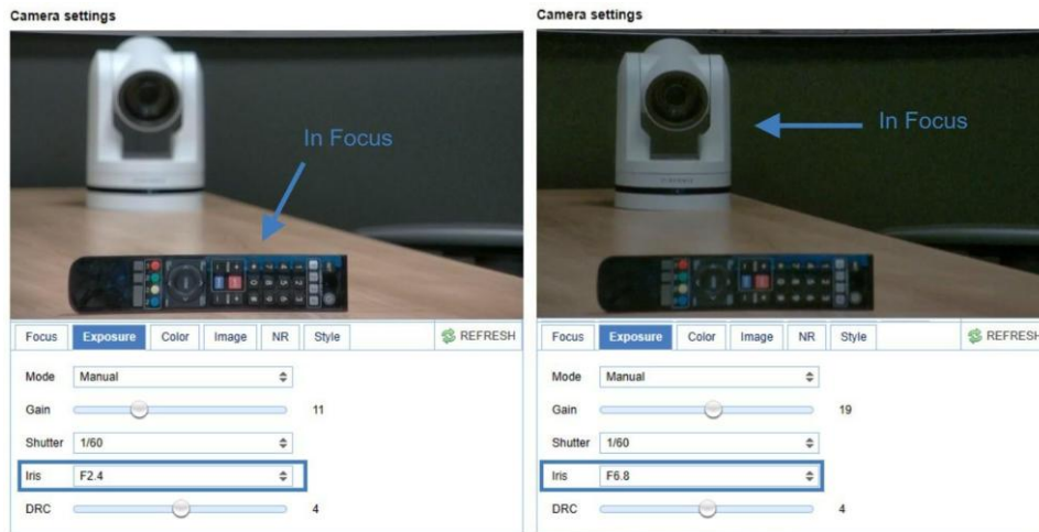
Figure 27: Exposure > Manual with Iris F2.0 (left) and Iris F6.8 (right)
