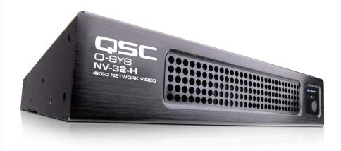
The NV-32-H (Core Capable) is a multipurpose, software-configurable video endpoint native to the Q-SYS Ecosystem that offers two distinct operating modes to choose between, based on the needs of the application.
