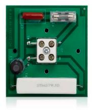
The PTL-1 is a Q-Sys accessory that provides an end-of-line 22 kHz impedance soak for 70/100V loudspeaker circuits. Used in combination with a QSC DataPort-equipped amplifier or CXD platform amplifier, the PTL-1 becomes a vital component for monitoring of a distributed loudspeaker line.
