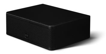
The Venu 208i is an ultra-compact self-powered double 8" subwoofer, capable of powering up to four mid-high enclosures, including Cyclone 4, Cyclone 55 and Indigo 6s from its built-in 600 Watt amplifier module. Providing a frequency response of 42 Hz – 120 Hz ±3 dB and a continuous output of 119 dB, peaking at 125 dB, the Venu 208i will provide flawless bass to any commercial/residential applications.
