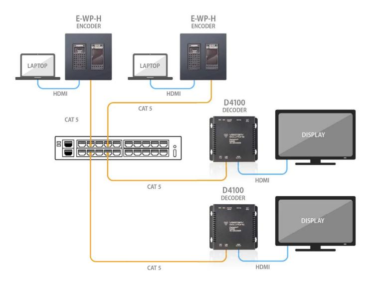
Figure 6. Many Sources to Many Displays Diagram
