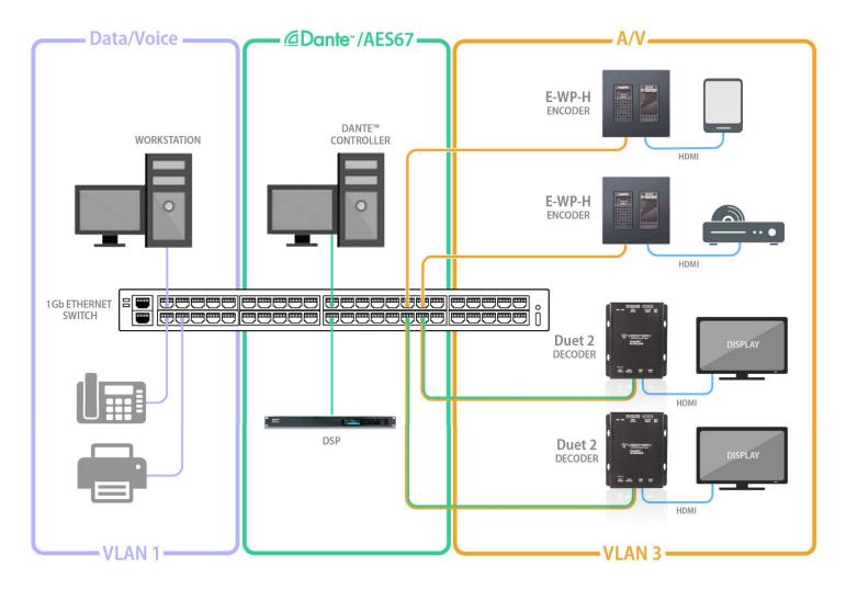
Figure 1. Converged Network Diagram
