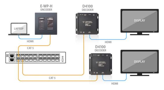
Figure 5. One Source to Many Displays Diagram
