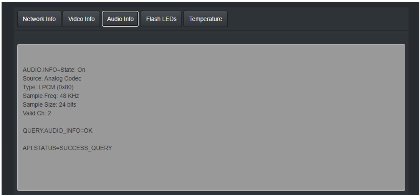
Displays the current audio source codec, type, sample frequency, and sample size information.
