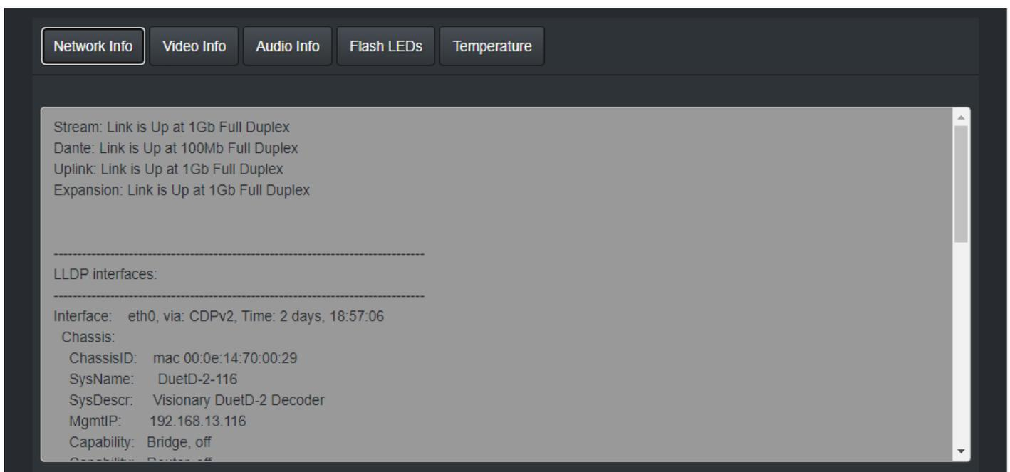
Displays the current network link speed for Stream and Uplink port. In addition, the network info displays local and neighbor LLDP information.
