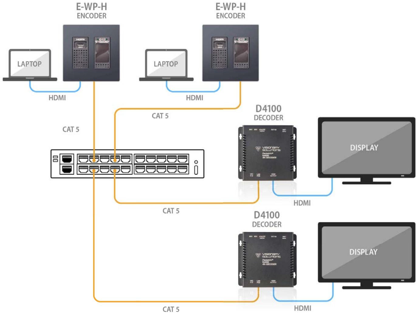
Figure 6. Many Sources to Many Displays Diagram
