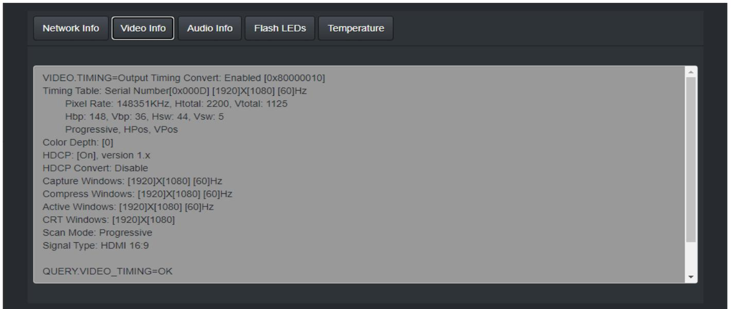
Displays the current video information, containing but not limited to resolution, refresh rate, scan mode, and HDCP.
