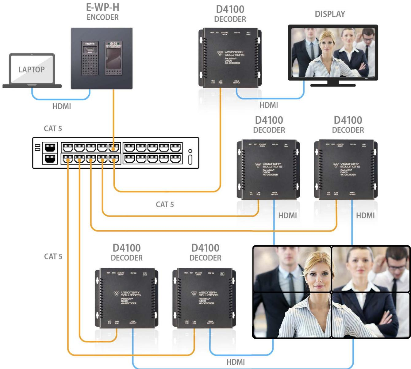
Figure 8. Video Wall Diagram
